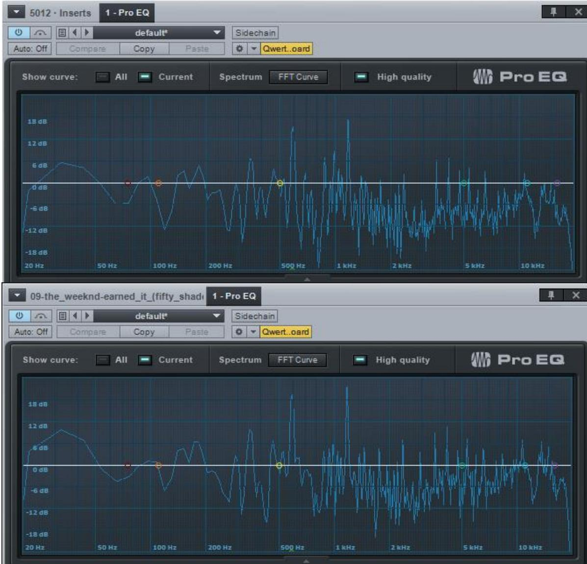
Overall, the frequency outputs are similar. One cannot tell if there is compression going on through the 5012 or not, however the peaks between 500 Hz and 1 kHz are noticeably shorter on the 5012's frequency spectrum compared to the original source audio. An interesting thing to point out is that there are no other glaring differences.
