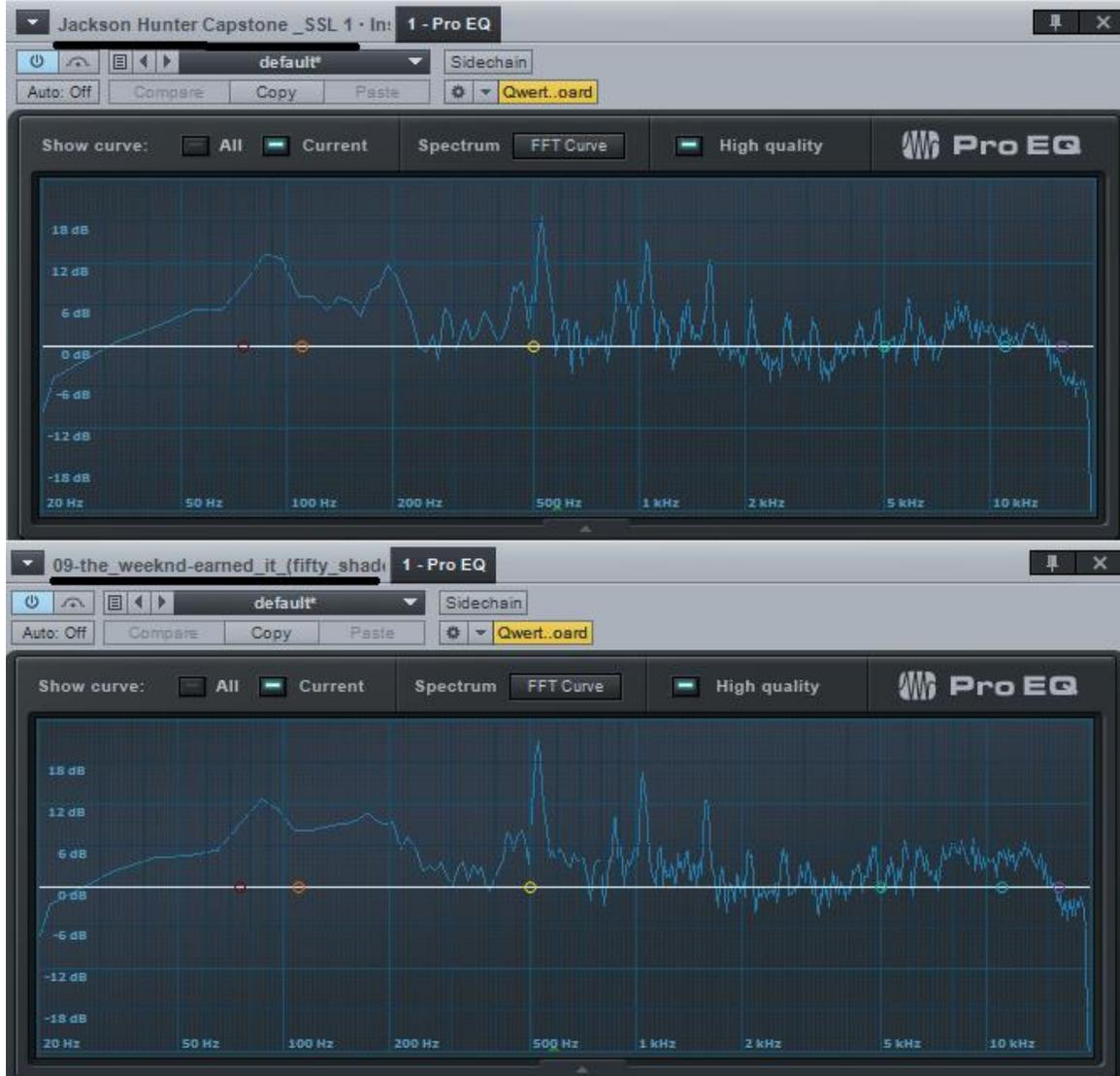
As one can see from the graphs above, the frequency outputs are strikingly similar, only differing in a few subtle areas. These slight differences can most likely be entirely attributed to the lapse in timing between screenshots. In conclusion, the Millennia STT-1 Origin vacuum tube has done nearly an identical job of replicating The Weeknd’s hit song, “Earned It.”
