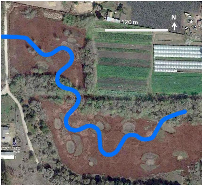
Figure 35: Approximately-scaled planform of a restored river channel across the southern and northern floodplains using design elements from table 8. Design is plotted on aerial photograph showing pond locations. Depending upon the final channel placement, ponds located near the channel should be decommissioned.
