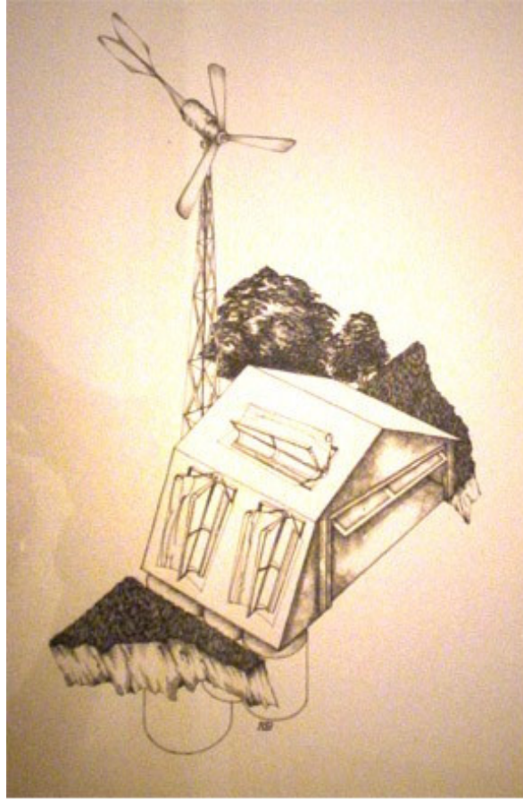
Figure 2 My first energy invention - a pre-fabricated garage with solar parabolic troughs, windmill, bio-digester, and high-temperature thermal energy storage (1974)
