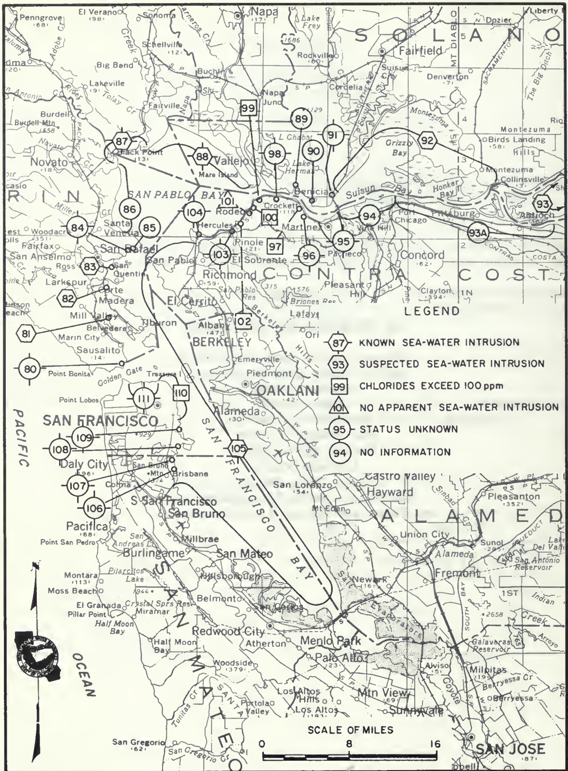
Figure 17. STATUS OF SEA-WATER INTRUSION, SAN FRANCISCO BAY AREA COUNTIES 1970-1971
