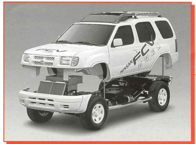
The Nissan Xterra fuel cell vehicle mockup features a full-size display of the fuel cell vehicle propulsion system.
