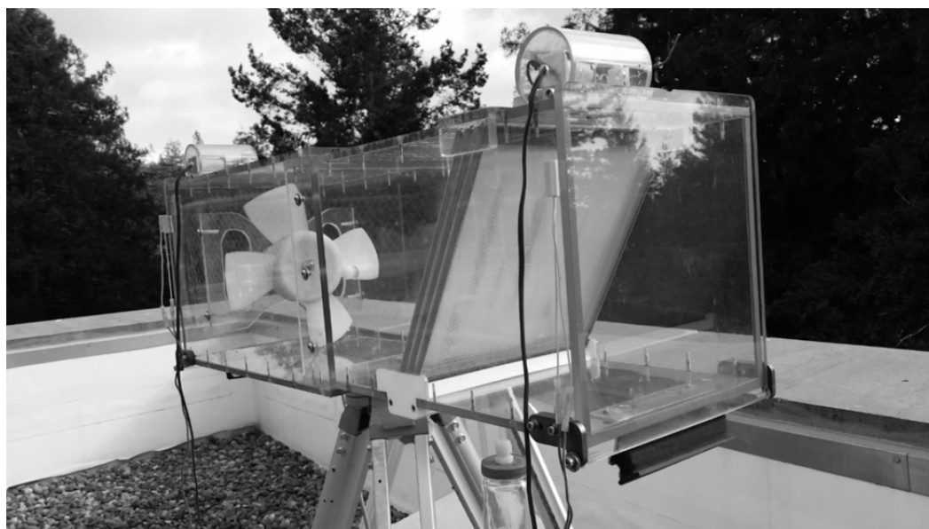
Fig. 1. The UCSC–built active fog water collector shown at a rooftop location on the UC Santa Cruz campus. Three strand frames with 0.508 mm diameter Teflon strings were used to collect fog droplets. The front and back doors were set under tension and popped open when the solenoid pull was engaged, shown at the top of the collector under a weather-protecting dome. The front and back reed-switch door sensors are also visible which prevent the fan from operating if the doors fail to open.
