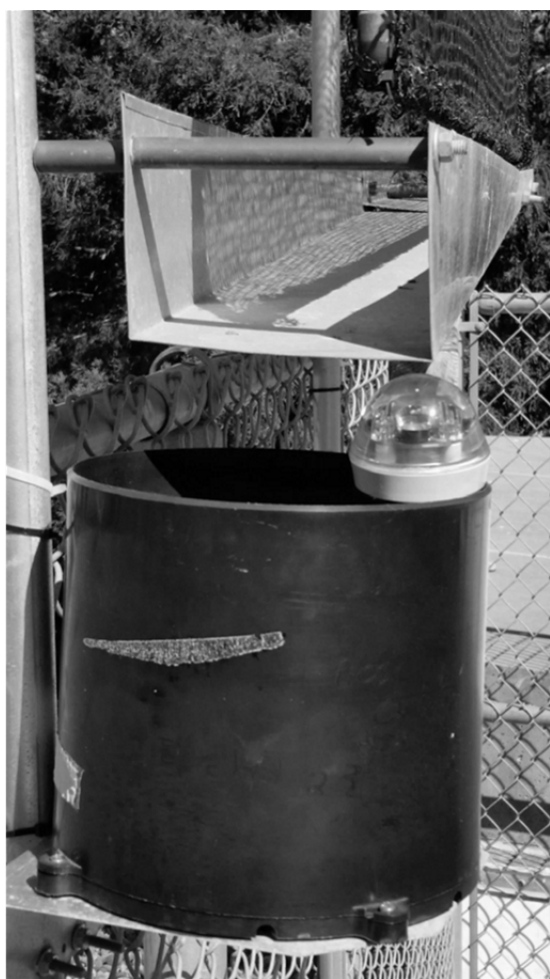
Fig. 2. Optical rain sensor (ORS) (RG-11) positioned at the terminus of the drip tray of the standard passive fog collector, and above the tipping bucket (TB) rain gauge. The drip tray is slanted downward slightly to the right so each drop exits the drip tray at the right-most corner and rolls across the ORS. There is a gap on the right side of the base of the ORS so that all droplets rolling off the ORS are collected in the TB.
