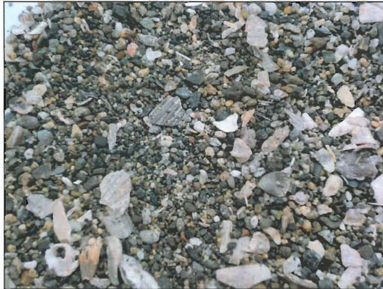
Figure 4-30 Example of sediment sample collected in Boundary Pass. Sample is coarse-grained sediment from the trough of a bedform field collected by the Geological Survey of Canada (GSC).
