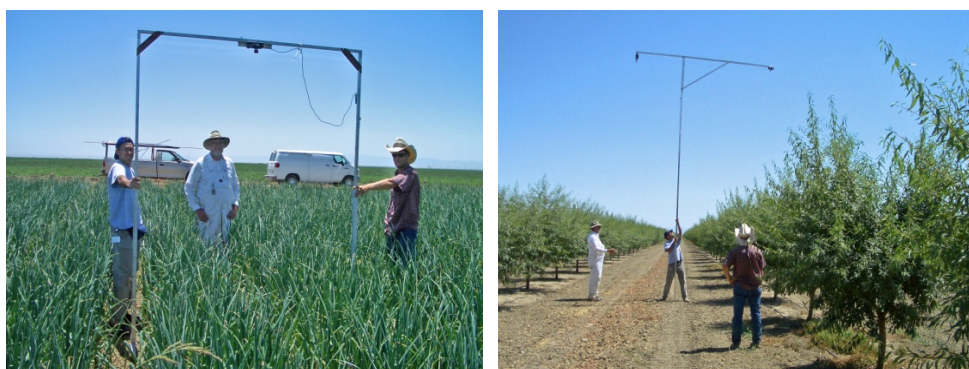
Figure 2. Measurement of green fractional cover ( F_c ) for low and high stature crops using multispectral camera.
