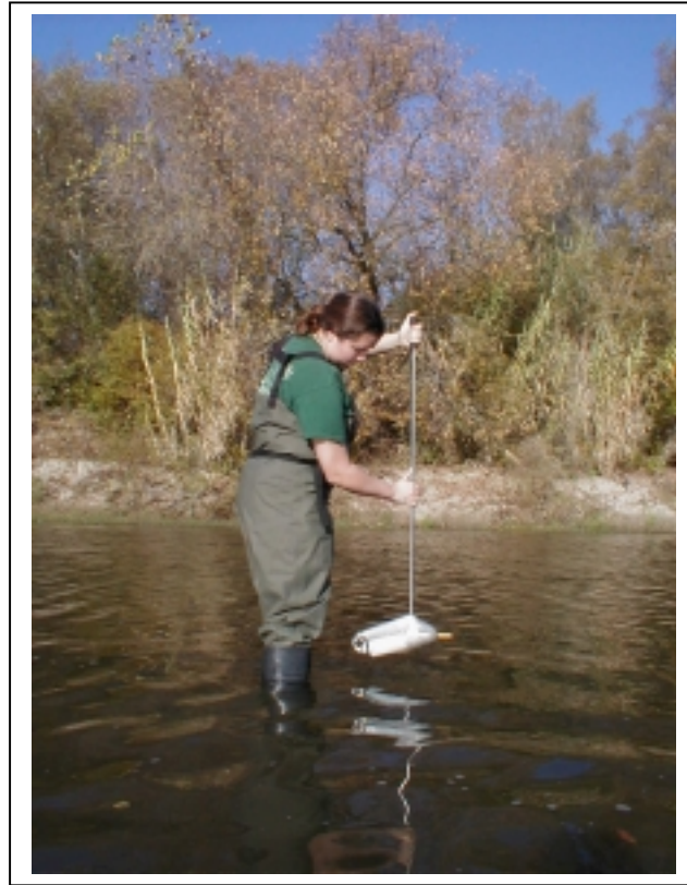
Figure 3: TSS sampling using a DH-48 instrument
