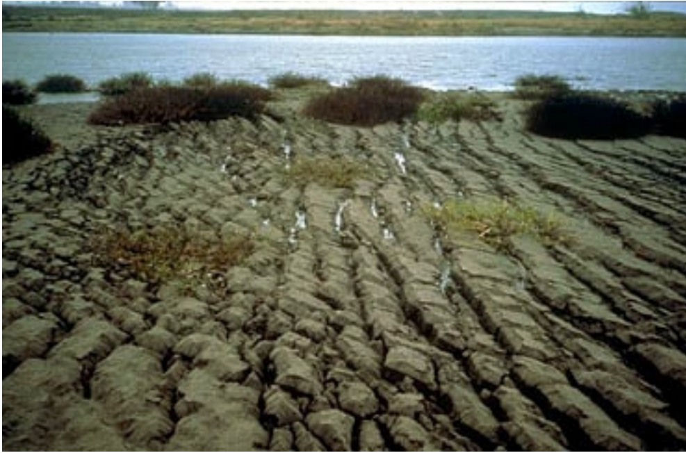
Liquefied ground near Moss Landing after the 1989 Loma Prieta Earthquake
