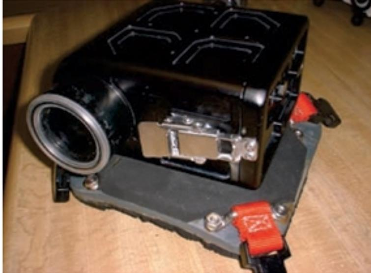
Figure 2: Waterproof camera housing
