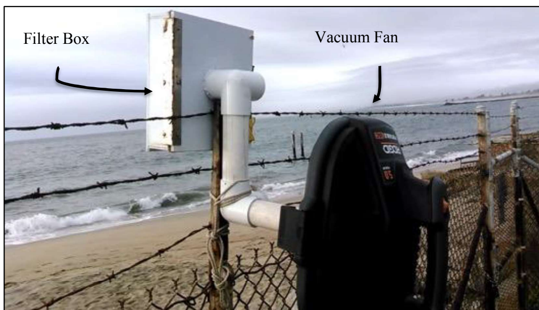
Figure 19. Aerosol collection module (used in aerosol generator) configured for sea spray collection.
