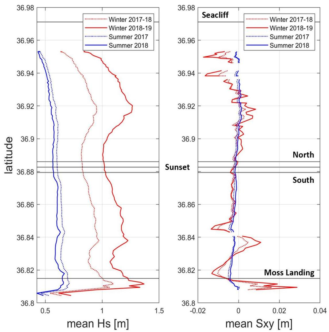
**Figure 13:** Averaged significant wave height (Hs) and alongshore radiation stress (Sxy) in the northern Monterey Bay. Winter (Nov, Dec, Jan) averages are shown in red and summer (Jul, Aug, Sep) averages in blue. The North and South horizontal lines denote the alongshore stretch of beach used to calculate shoreline change due to alongshore sediment transport in the present study.
