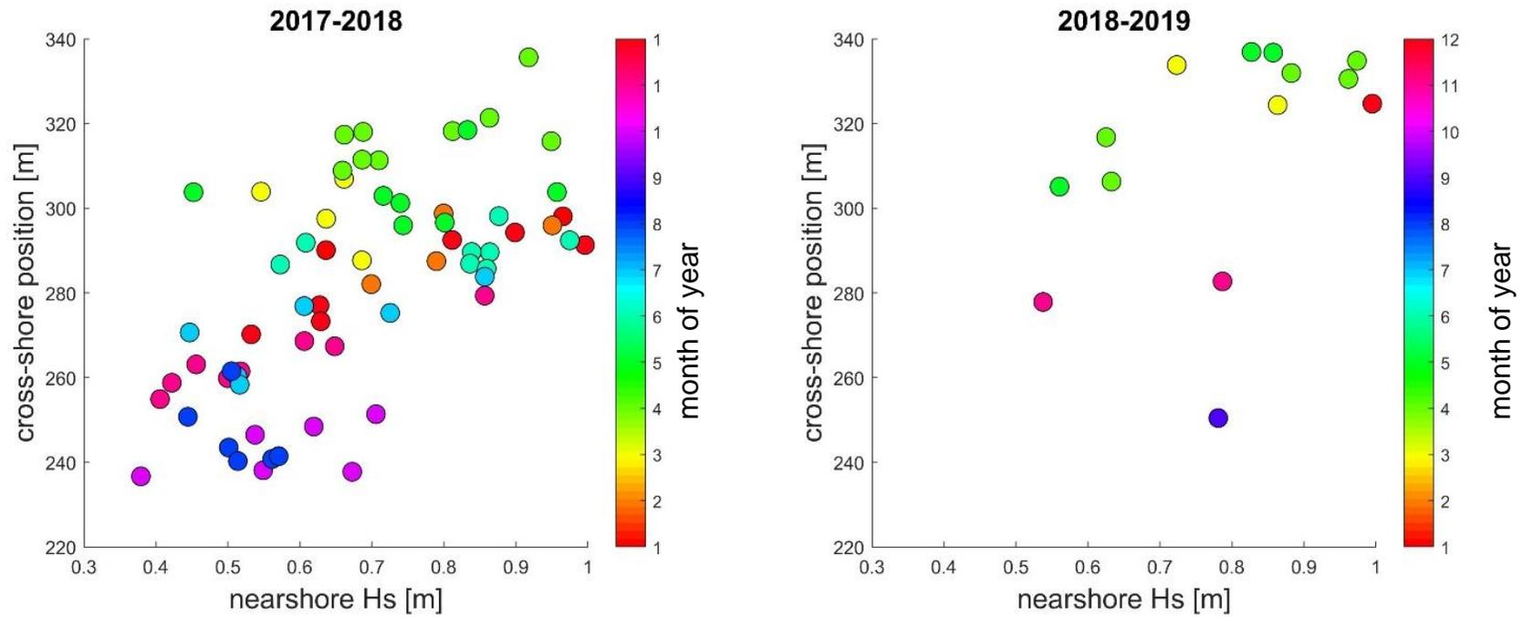
**Figure 7:** Cross-shore sandbar position vs. nearshore significant wave height (Hs) for year 1: October 2017 – August 2018 (left) and year 2: September 2018 – April 2019 (right). Data is colored by month of year (January = 1, February = 2, etc.). Sandbar position was positively correlated with wave height, the overall  $r^2 = 0.40$  for all sandbar observations.
