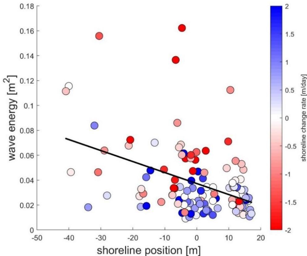
**Figure 9:** Shoreline change rate  $\frac{dS}{dt}$  between consecutive shoreline observations and averaged wave energy at Sunset State Beach. The black line shows the linear fit ( $r^2 = 0.25$ ) used to determine initial parameters (y-intercept  $b = 0.037m$ , slope  $a = -0.00081 m^2/m$ ). The black line represents an estimated equilibrium state where no shoreline change is expected according to shoreline position and wave energy.
