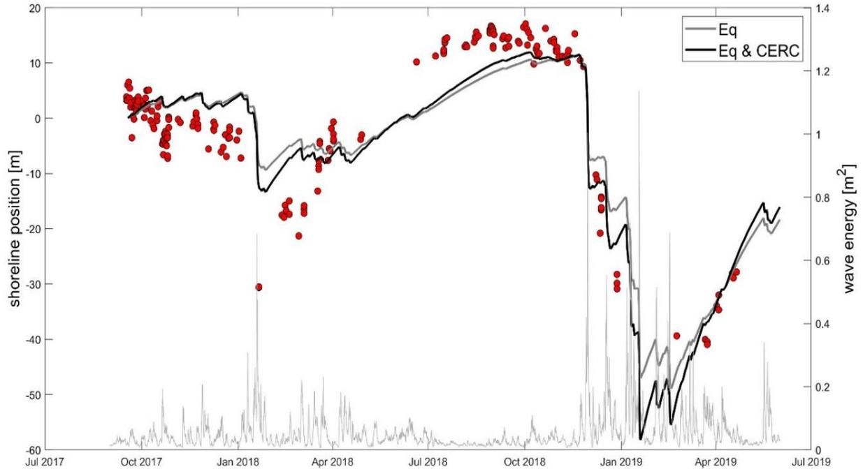
**Figure 10:** Equilibrium shoreline model predictions using optimized parameters for image mapped shorelines from fall 2017 to spring 2019. Hourly model predictions are shown in black for the Equilibrium model expanded with CERC and grey for the equilibrium model alone. Shorelines mapped by imagery are shown by red points. Wave energy is shown in light grey according to the right axis.
