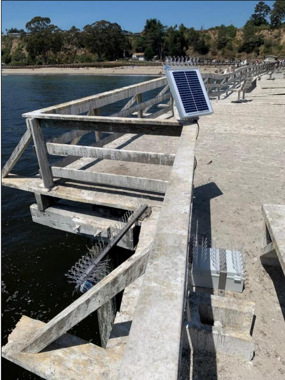
**Figure 14:** Radar water level sensor at Seacliff State Beach.
