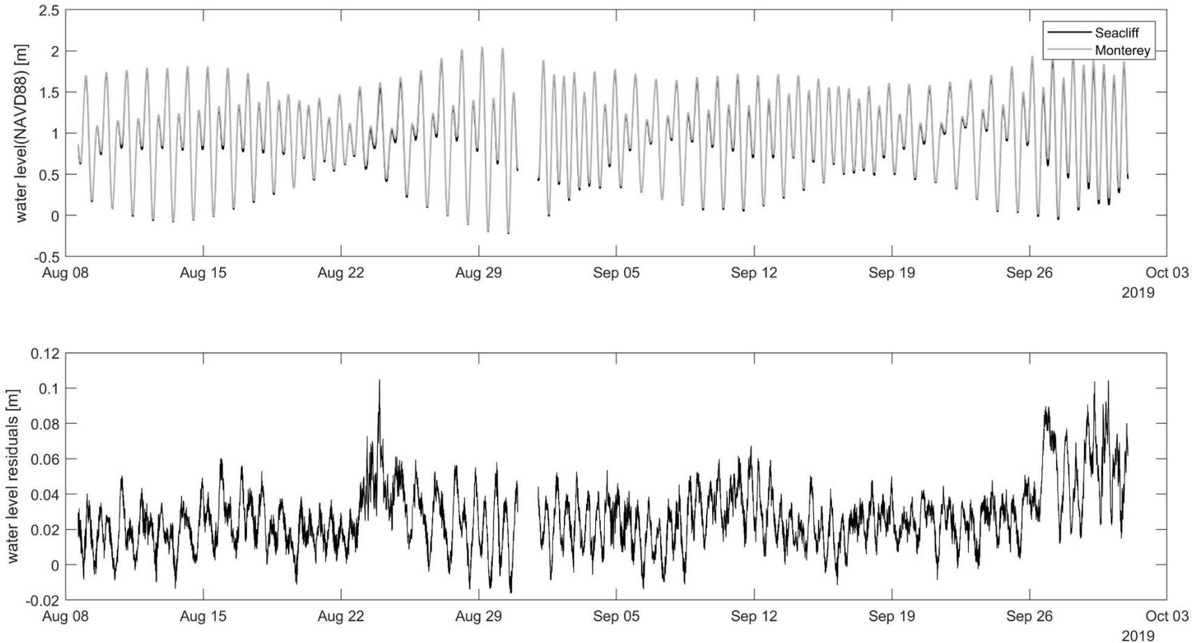
**Figure 15:** Comparison between total water levels at Seacliff State Beach and the Monterey Wharf. Water levels in the top panel are georeferenced to NAVD88; a 0m water level corresponds to the elevation of NAVD88. Positive residuals in the bottom panel indicate times when the Monterey tide gauge reported higher water levels than those in Seacliff. GPS surveying and data processing was performed by Joshua Logan of USGS.
