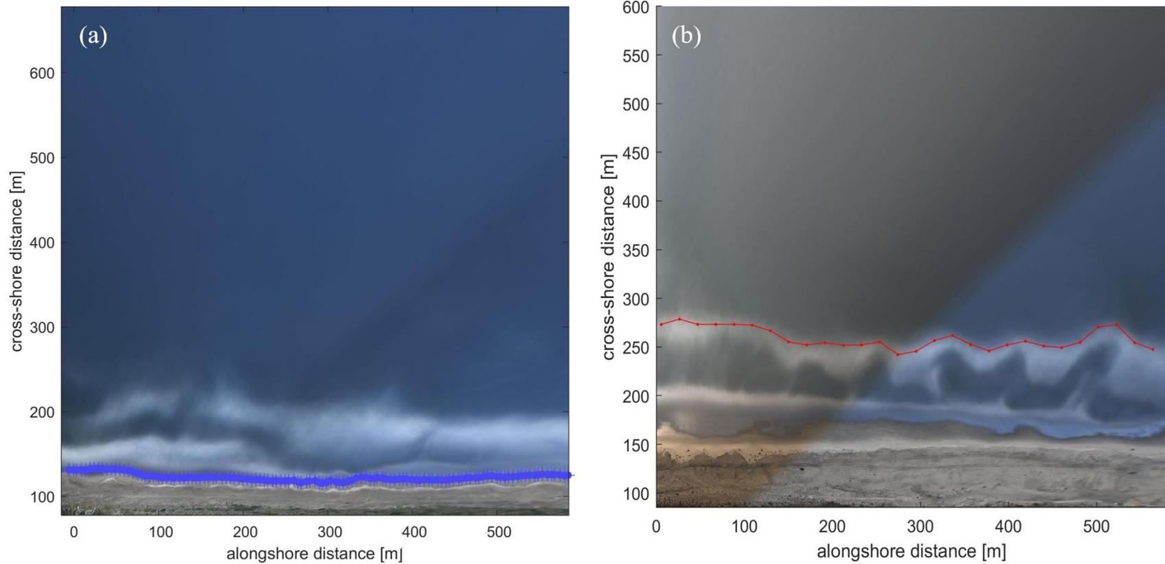
**Figure 4:** Example of shoreline (a) and sandbar (b) position mapping using rectified time exposure image products. The cross-shore shoreline position was mapped every 5 meters alongshore (cross hatches along blue line), while the cross-shore position of the outer sandbar was mapped every 10m alongshore (points along red line).
