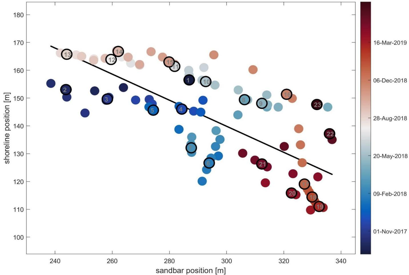
**Figure 8:** Weekly shoreline vs. sandbar positions at Sunset State Beach colored,  $r^2 = 0.57$  and linear slope is  $-0.47\text{m}$  (black line). Since shoreline and sandbar positions were not observed at the same time during the study period, the time series were synchronized and interpolated to display weekly observations and are colored by time. Monthly positions are outlined in black and numbered beginning at 1 in October 2017 (darkest blue).
