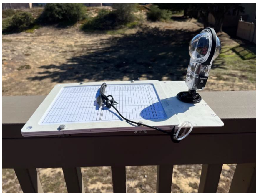
Figure 2 – Insta360 X2 attached to a PVC dive slate with a datasheet. This configuration allowed UVC and 360° video data to be collected simultaneously.
