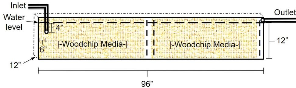
**Figure 2.** Cross section of a bioreactor channel with woodchips
