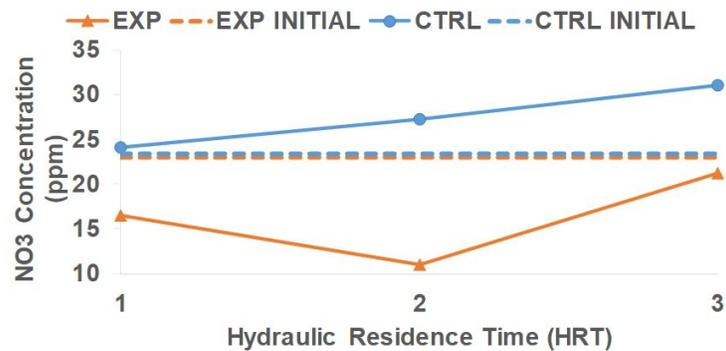
**Figure 3.** Nitrate concentrations of experimental and control bioreactors as samples were collected at different HRTs from one experiment run.
